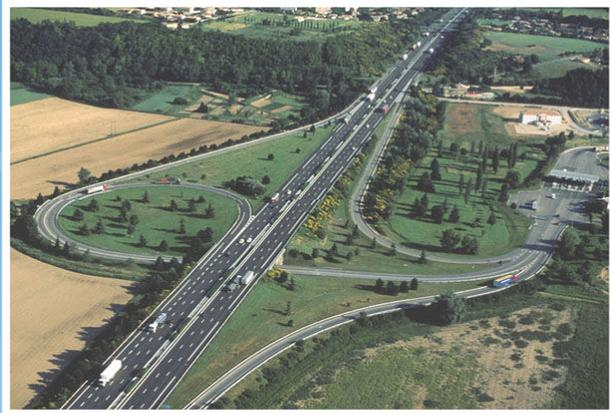
Motorways are characterised by dual carriageways for the two directions of flows (completely separated by a central reserve), the lack of intersections at level, proper lanes for on/off merging and the presence of grade-separated interchanges
